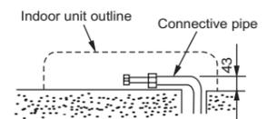
3. Fix the end of the connective pipe. (Refer to Tightening Connection in REFRIGRANT PIPING CONNECTION)
