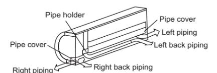
1. For the left-hand and right-hand piping, remove the pipe cover from the side panel.
