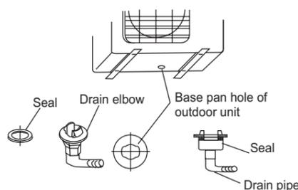
Fit the seal into the drain elbow, then insert the drain elbow into the base pan hole of outdoor unit, rotate 90° to securely assemble them. Connecting the drain elbow with an extension drain hose (Locally purchased), in case of the water draining off the outdoor unit during the heating mode.
