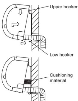
1. Pass the piping through the hole in the wall.
